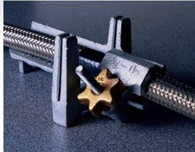
Place the conduit along the vice body and tighten the clamp. Holding the conduit and integral handle together, insert a hacksaw blade into the guide and cut. For braided conduit, wrap adhesive tape around the cutting point to secure braid. Remove tape after cutting.
