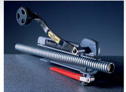
Adjust the clamping pin so that the conduit is just held in the recess. Squeeze the lever and body whilst rotating the cutting blade. When the blade appears on the inside of the conduit, release the pressure and remove the conduit. A simple twist will then separate the two parts. Where the conduit is covered, the covering can be cut prior to separation. Spare blades are available.
